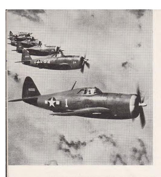
THE REPUBLIC P-47 THUNDERBOLT. The Thunderbolt is 35 feet long and 41 feet from wing tip to wing tip. It weighs nearly seven tons, as much as 5 average automobiles. Yet it is flown easily by one man, who operates all
